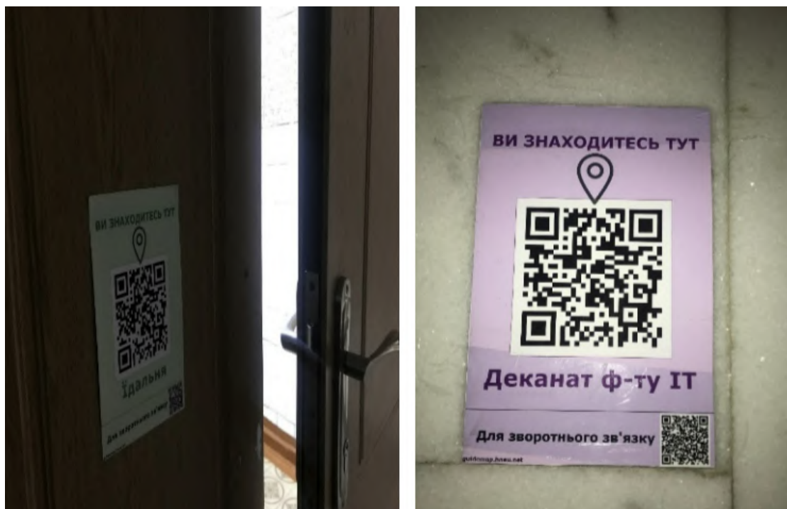
Figure 9: QR code labels placed in the relevant locations of the university premises which enable university visitors to access the navigation system, use it, and give a feedback.
