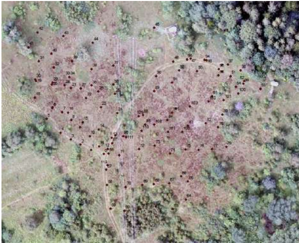
Fig. 8. Orthophoto map of mountain part of Skhidnytsya created in 2018 overlapped with check point network obtained by GNSS-survey (all data are referenced to the coordinate system WGS84 and the Baltic Heights)
