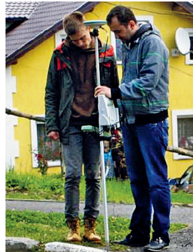
Fig. 4. The process of obtaining the coordinate of ground control points by GNSS method
