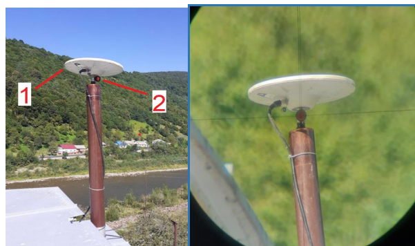
Fig. 8. Continuous GNSS station TERE 1 – GNSS antenna, 2 – reflector
