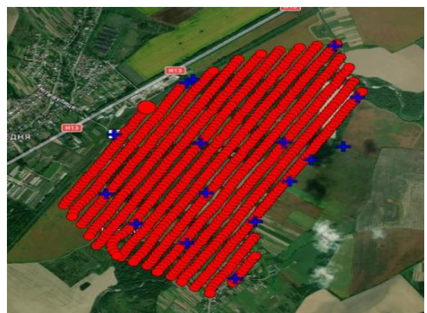
Fig. 4. Scheme of the location of the centers of projections of digital images and points of geodetic base 2021
