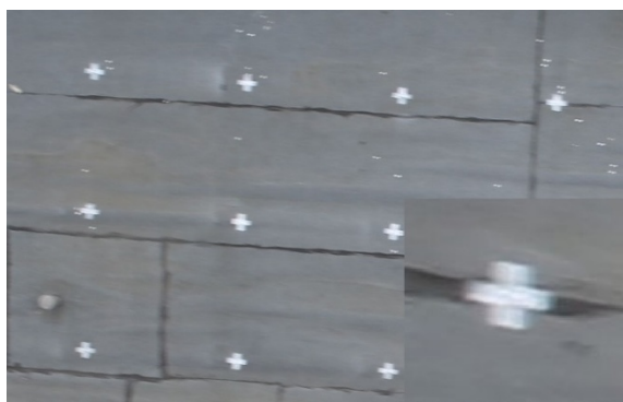
Fig. 12. Linear image motion during aerial survey from the octocopter DJI S1000
