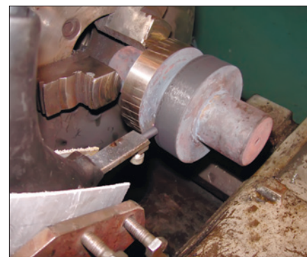
Fig. 2. EEAC-treatment using the turning machine
