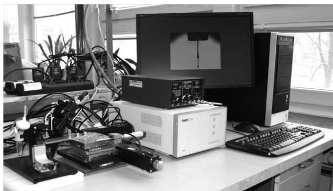
Fig. 1. Ink-jet printer constructed in Tele- and Radio Research Institute [3]
