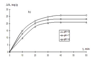
**Figure 3** – Dependence of the degree of saturation of the sorbent iron ions (a) and zinc (b) from time to time at different pH values
