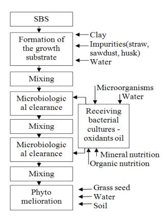
Figure 1 – Process of manufacturing operations solid bottom sediments disposal.
