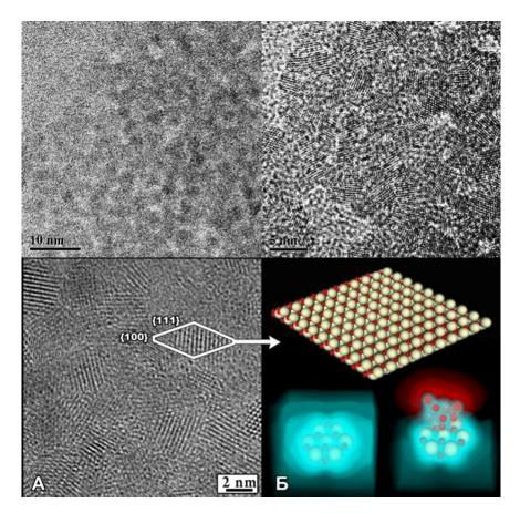
F i g. 2. HRTEM of CeO<sub>2</sub> nanoparticles in citrate-stabilized sol (top, bottom "A") and Virtual NanoLab model of citrate- stabilized nanoceria (bottom "Б")
