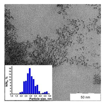
F i g. 1. Micrograph of CeO<sub>2</sub> nanoparticles in citrate-stabilized sol. Inset: particle size distribution according to TEM data
