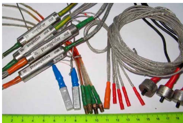
Fig. 6. Pressure and acceleration sensors
