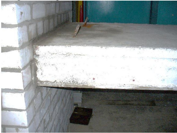
Fig 11. The upper surface of slab 11 about pinch after the test
