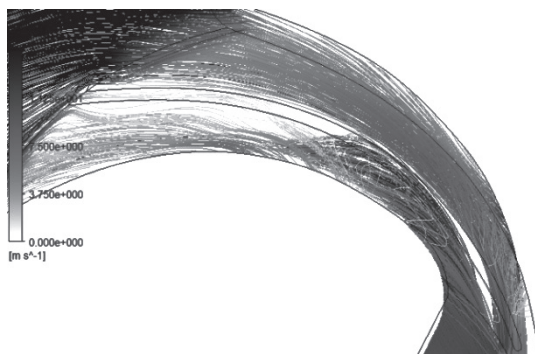
Fig. 6. The current flow lines in the impeller channel with the outlet width of 92 mm in 0.5 Q_{opt} operation mode
