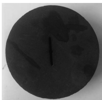
Fig. 3. SNBD Specimen made by high-pressure water jet method
