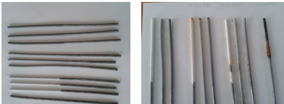
Fig. 5. Steel bars before and after testing in different media
