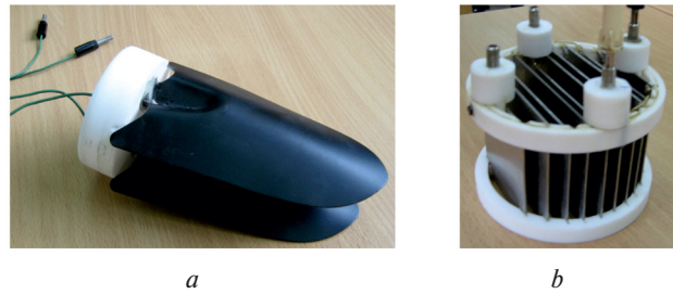
Fig. 3. Capacitance instrument transducers: a – T1 with two teflon-coated plates; b – T2 with multiple epoxy-varnished plates
