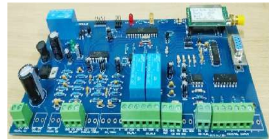
Fig. 2. Structure and PCB of Sensor station: a – block diagram of SSs; b – realistic circuit board of sensor stations
