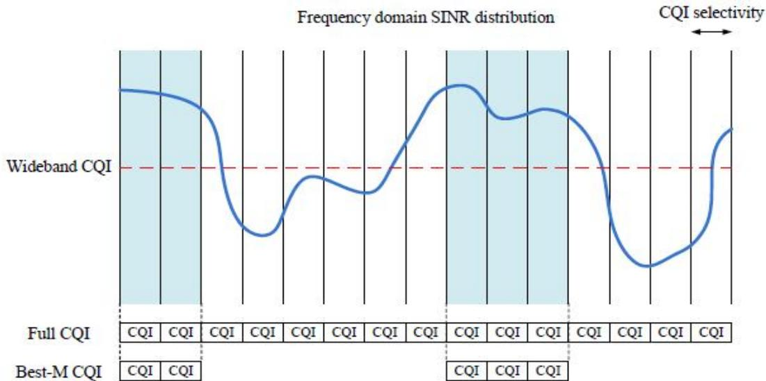
Fig. 1: Illustration of the three CQI reporting methods
