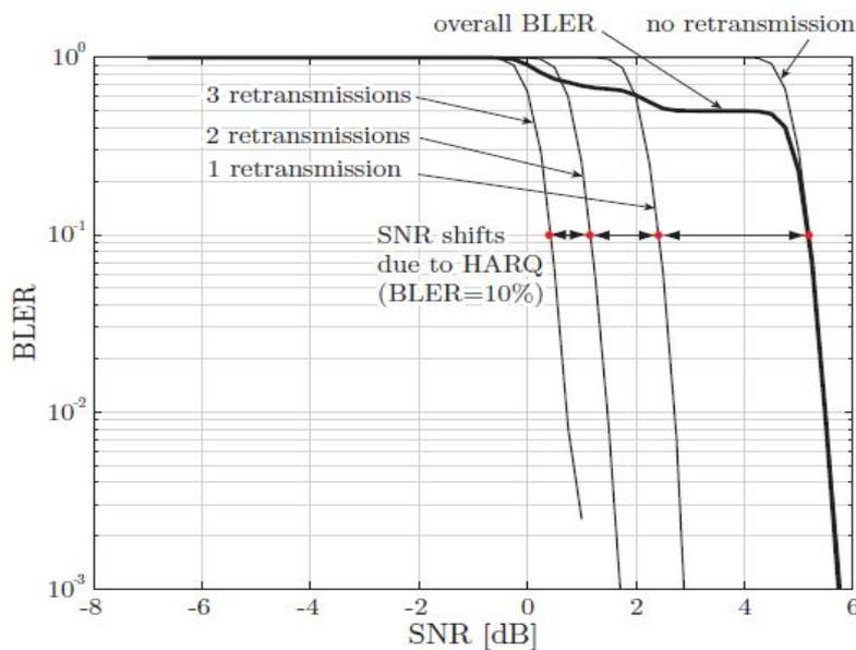
Fig. 3. Resulting BLER at CQI=7 for different number of allowed retransmissions
