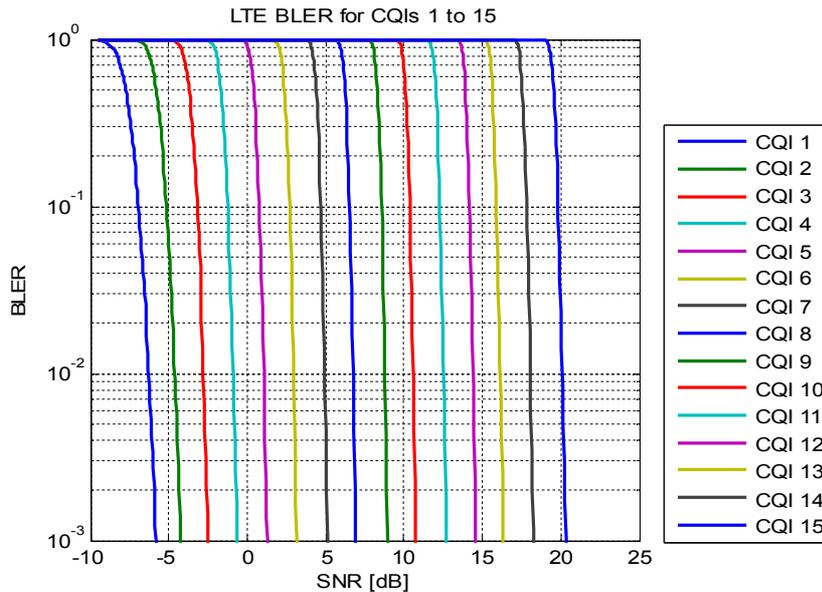
Fig. 2. BLER curves obtained using AWGN for all 15 CQI values. From CQI 1 (leftmost) to CQI 15 (right most)
