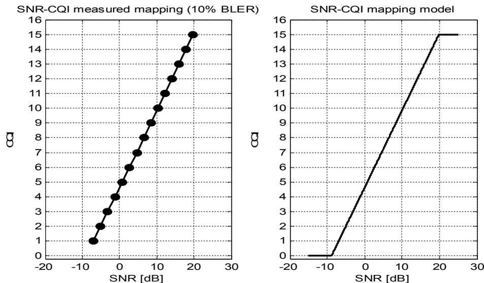
Fig. 4. CQI mapping. BLER=10% points from the BLER curves (left) and SINR-to-CQI mapping function (right)
