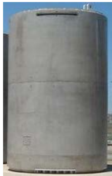
Fig. 7. VSC-WWER at the moment of installation in storage
