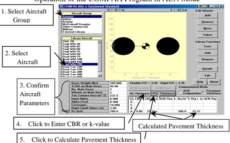
Operation of the COMFAA Program in Pavement Thickness Mode
