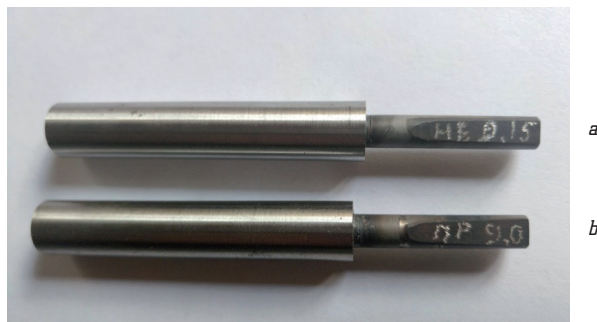
Fig. 1. Caliber for 9 mm pistol PM: a – go gage; b – no-go gage
