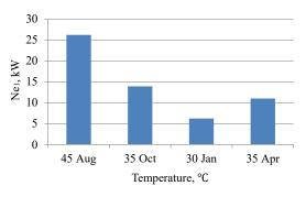
Fig. 6. Dependence of the power Ne1 on the ambient temperature
