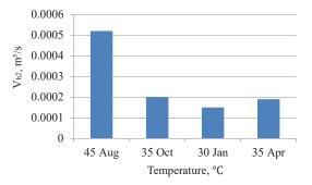
Fig. 7. Dependence  $V_{h2}$  on the ambient temperature
