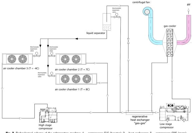
Fig. 3. Technological scheme of the refrigeration machine: 1 – compressor CLS (booster); 2 – heat exchanger; 3 – compressor CHS (main); 4 – gas cooler; 5, 7, 9 – throttle valves; 6 – liquid separator; 8, 10 – air coolers
