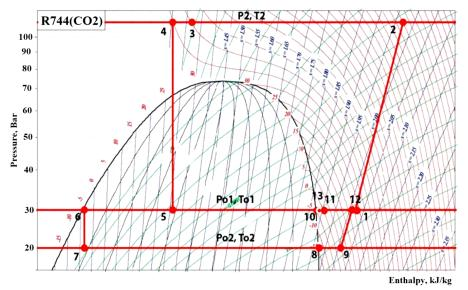
Fig. 4. Thermodynamic cycle in diagram p-h
