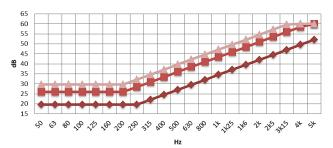
Fig. 2. Sound insulation frequency response for aerated concrete walls with density 400 kg/m<sup>3</sup> and different thicknesses: → - 100 mm; → - 200 mm; → - 300 mm
