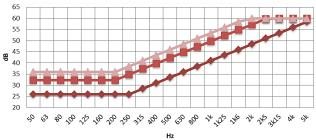
2.1.3. Gypsum wall with a layer. Two-layer construction such as two sheets of drywall, mineral wool, two sheets of drywall, taken from calculates based on [4].
