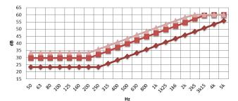
Fig. 3. Sound insulation frequency response for aerated concrete walls with density 600 kg/m<sup>3</sup> and different thicknesses: → - 100 mm; → - 200 mm; → - 300 mm
