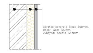
Fig. 7. Structure of a sample
