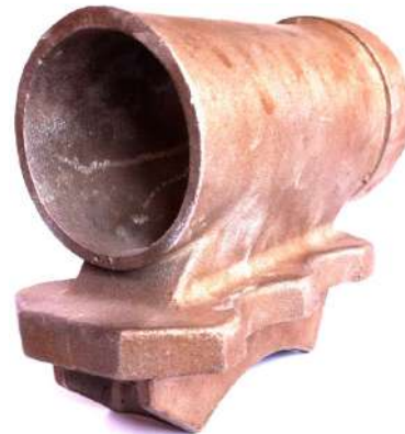
Fig. 2. Casting of high quality in terms of continuity without gating system
