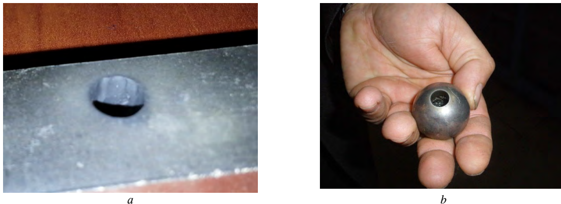
Fig. 5. Obtaining quality holes (a) and defective holes (b) in hard-alloy workpieces
