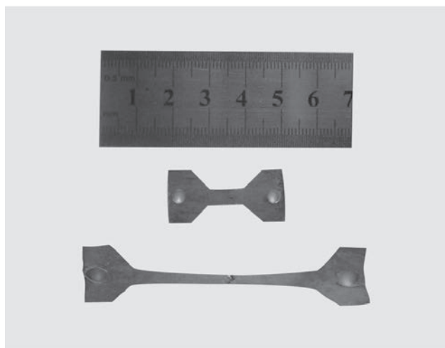
Fig.4. General view of the specimen of alloy 1933, previously passed hot working, deformed to failure in mode of superplasticity in optimal conditions to 410% in comparison with the initial.
