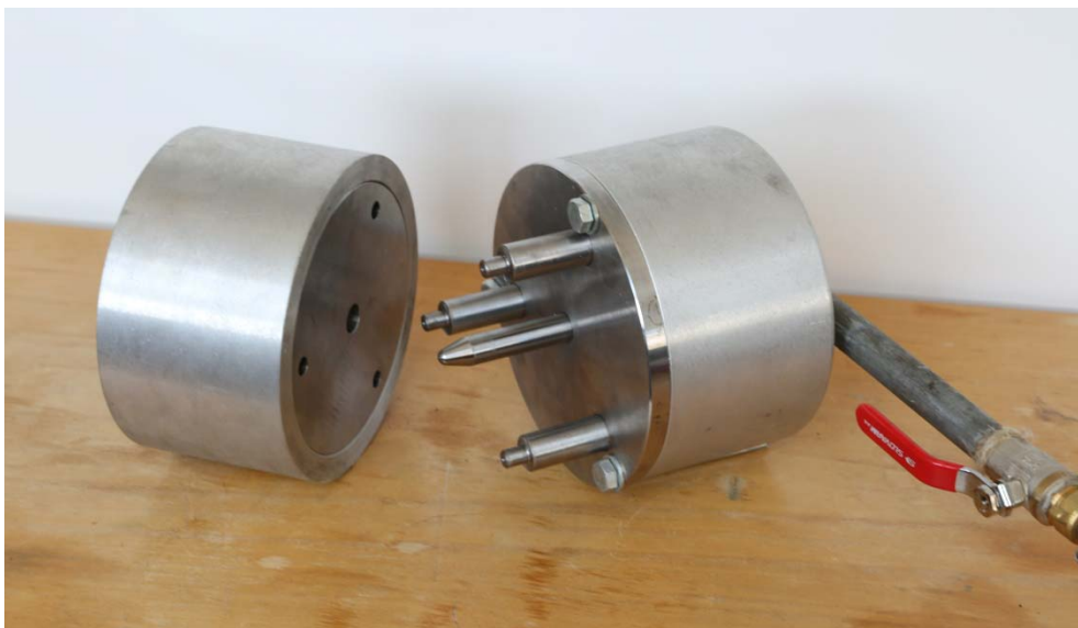
Fig. 7. Photograph of disassembled tool for rotary yields
