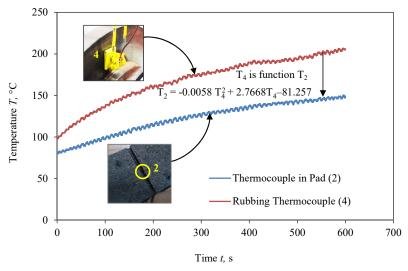
Fig. 5. Relation temperature between position 2 and 4
