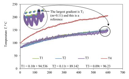
Fig. 4. Brake temperature detection results
