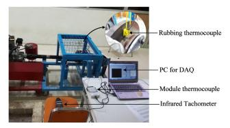
Fig. 1. Set-up experiment test rig
