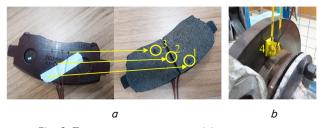
Fig. 2. Thermocouple sensor position: a – sensor thermocouple in Pad (position 1, 2, 3); b – rubbing thermocouple (position 4)
