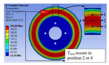
Fig. 3. Temperature rotor brake contours
