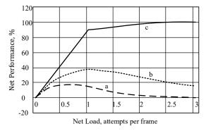
Fig. 4. Graph of computer network performance for different access methods: a – ALOHA; b – discrete ALOHA; c – CAN
