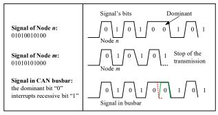
Fig. 2. Procedure for determining priorities during arbitration
