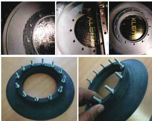
Fig. 11. Stages in flange reproduction and the obtained experimental samples
