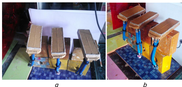
Fig. 2. The components of plotters glued (grey adhesive seam along the edges) by gypsum-epoxide (in this work, designated “ G_h ”): a – a side view; b – top view
