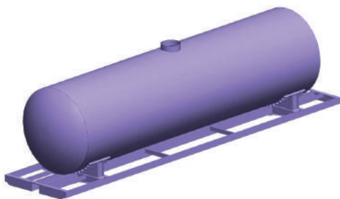
Fig. 2. A spatial model of the bearing structure of a tank car
