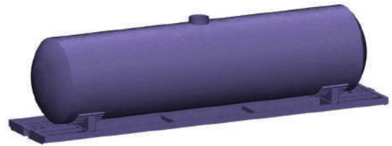
Fig. 9. A finite-element model of the bearing structure of a tank car
