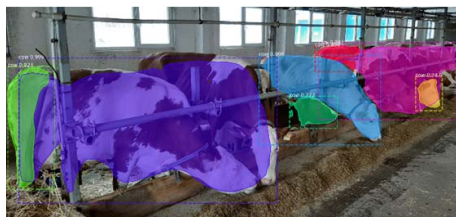
Fig. 11. Examples of false recognitions in real conditions: a – false detection; b – several animals were recognized as one
