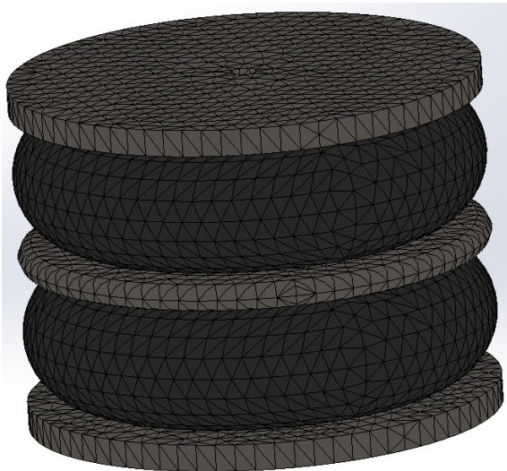
Fig. 3. A finite-element grid of the pneumatic spring in 3D format
