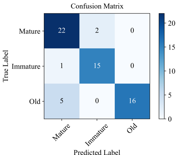
Fig. 6. Test result on Nvidia Jetson Nano using 100x100 input on CNN model with 4 Convolutional and 4 MaxPooling
