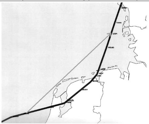
Fig. 2. ATS Routes Straightening within Free Route Airspace
