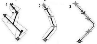
Fig. 4. Conventional routes compared to PBN-based routes:
