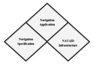
Fig. 5. Components of PBN Concept
