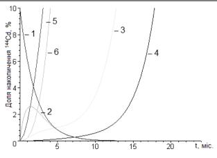
Fig. 4. Graphic of radioisotope <sup>114</sup>Cd accumulation in components of water ecosystems at  $C_{ac biota} = 0.8$ : 1 – accumulation of <sup>114</sup>Cd in box sewage waters a(t), 2 – accumulation of <sup>114</sup>Cd in box *surface waters* b(t), 3 – accumulation of <sup>114</sup>Cd in box *bottom sediments* c(t),
