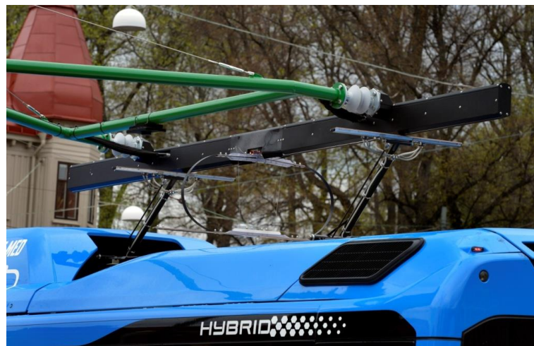
Rys. 6. System ACS (Automatic Roof-Top Connection System) zamontowany na dachu autobusu Volvo[2, 5]
