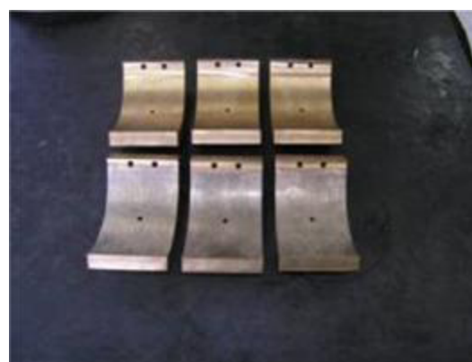
Fig. 3. The bronze pads of the sliding bearings
