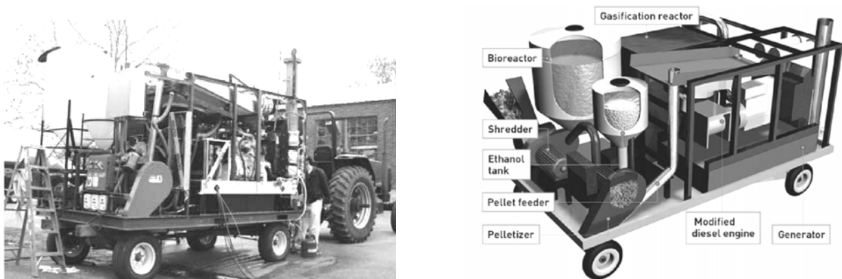
Fig. 2. Tactical garbage to energy refinery
