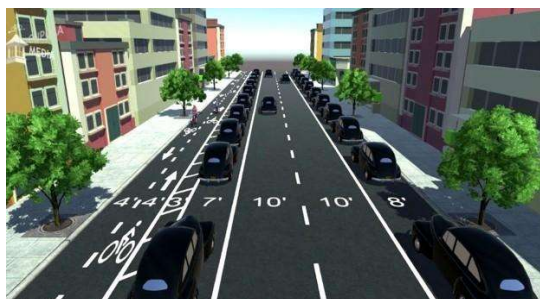
Figure 8 – Two lanes instead of three
