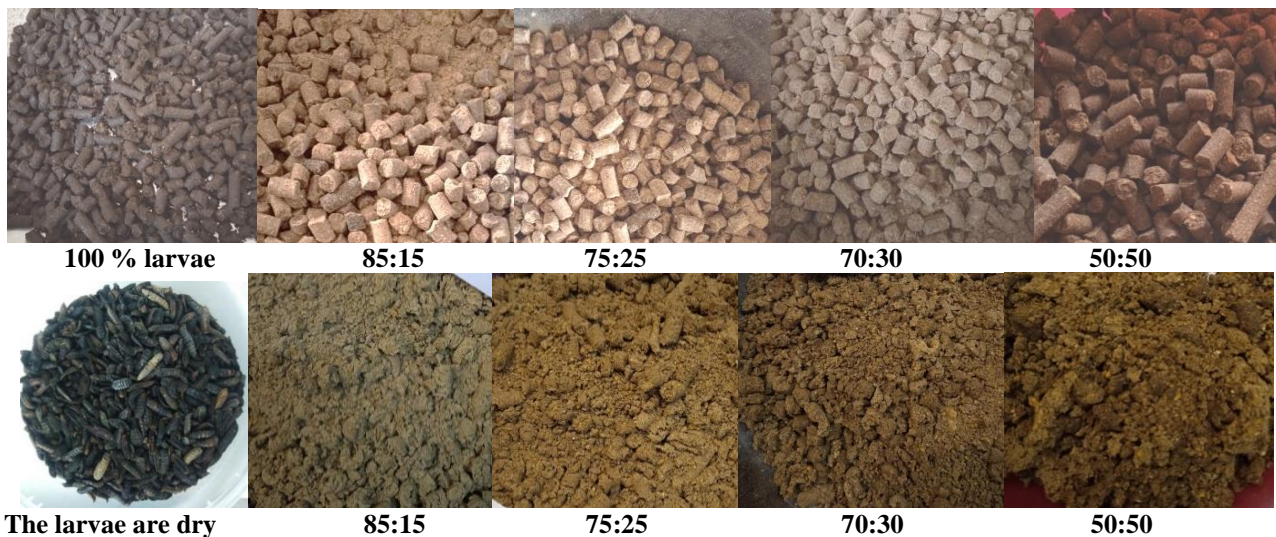
Fig. 4. Granulated and extruded mixtures of grain with larvae (maize grain:larvae)
