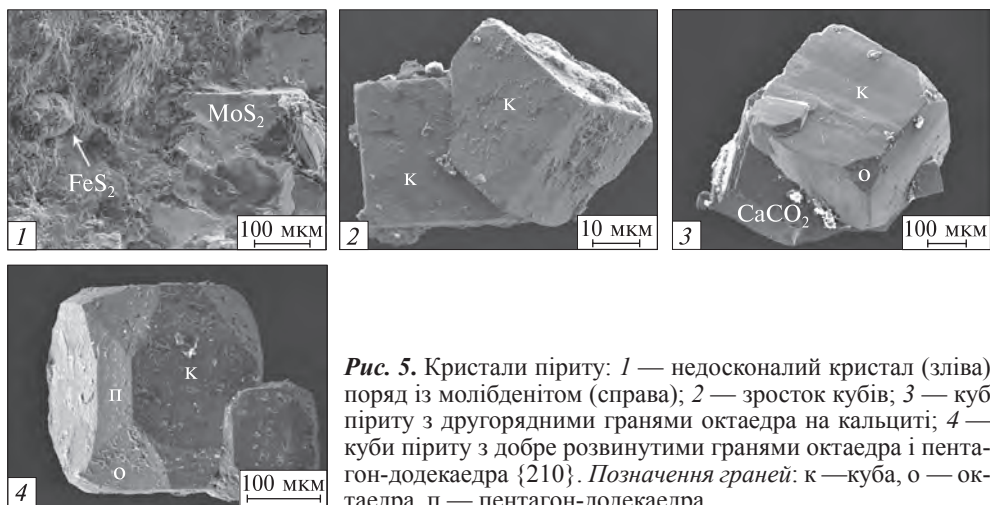
Fig. 5. Pyrite crystals: 1 — pyrite imperfect crystal in the rock (left) with molybdenite (right), 2 — aggregate of pyrite cubes, 3 — pyrite cube with minor octahedron faces on calcite, 4 — pyrite cubes with well developed faces of octahedron and pentagonal dodecahedron \{210\} . Mark faces: к — cube, о — octahedron, п — pentagonal-dodecahedron
