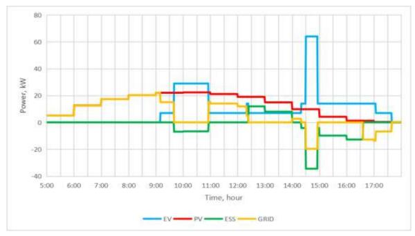
*Fig. 7.* Power dispatch in operating mode with optimization (summer) *Source:* compiled by the authors
