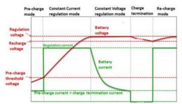
Fig. 2. Change in current and voltage when charging a lithium-ion battery according to the constant current / constant voltage rule Source: compiled by the [15]
