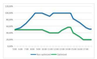
Fig. 8. Comparison of state-of-charge for modes with and without optimization in summer Source: compiled by the authors
