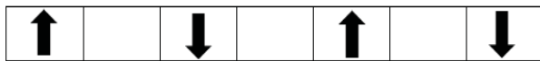
Fig. 3. Scheme of the magnetization system of the inductor by radially magnetized magnets
