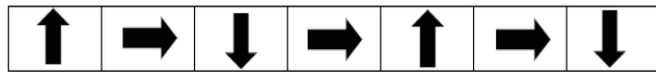
Fig. 4. Scheme of the magnetization system of the inductor by radially magnetized magnets
