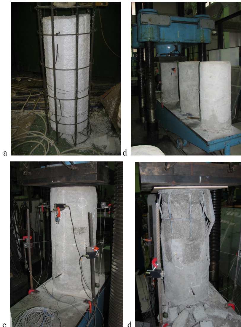
Fig. 3. Column fragment test: a – a framework for producing the column; b – ready columns before the test; c – alignment of sensors to determine the strain; d – a ruined column fragment
