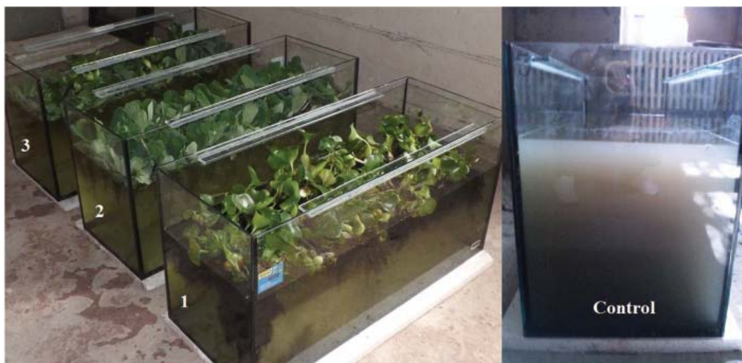
Fig. 2. Research scheme of hydrophyte systems operating regimes (from left to right): 1 — E. crassipes (Mart.) Solms — 100%; 2 — P. stratiotes L. — 100%; 3 — E. crassipes (Mart.) Solms — 50% + P. stratiotes L. — 50%; 4 — Control (without hydrocoles)
