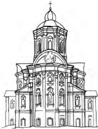
Fig. 14. A sample of the counter-apse triconch church: St. Michael's Church in the village Voronizh in Sumy region.
