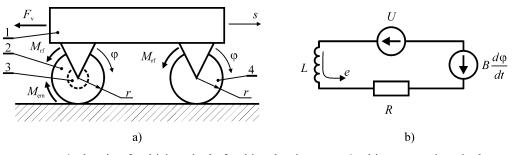
1 - housing; 2 - driving wheels; 3 - drive electric motors; 4 - driven supporting wheels
