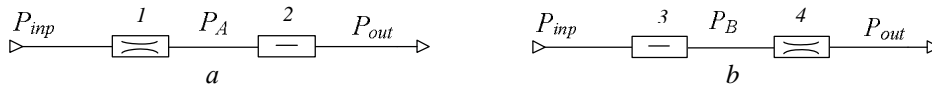
Fig. 1. Schemes of throttle dividers: a – turbulent-laminar divider; b – laminar-turbulent divider 1, 4 – turbulent throttles; 2, 3 – laminar throttles
