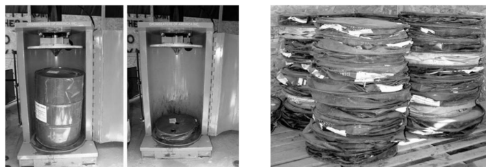
Fig. 3. The process of piercing, washing, and pressing of metal pesticide containers
